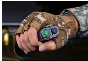
Battery level indication and low voltage warning.
